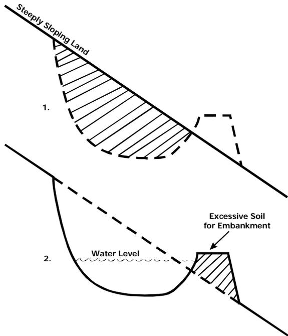
**Figure 3: Pond construction on steeply sloping land**
