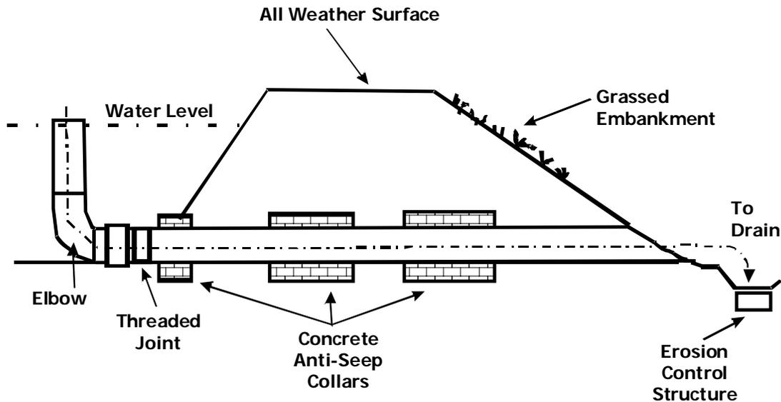
Figure 10: Cross-section of drainage system and pond embankment
