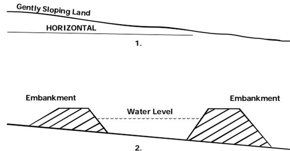
**Figure 5: Pond construction on gently sloping land**
