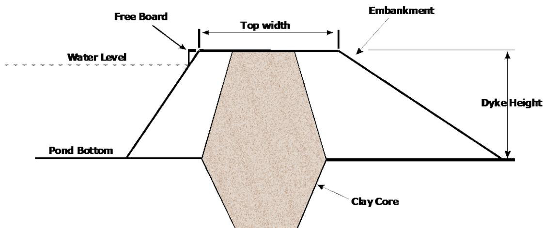
Figure 9: Typical cross-section of pond embankment
