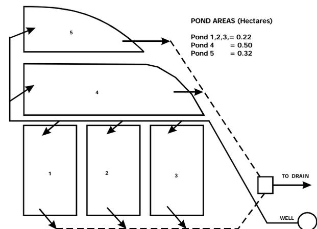
**Figure 7: Layout and design of ponds to fit existing land shape**
