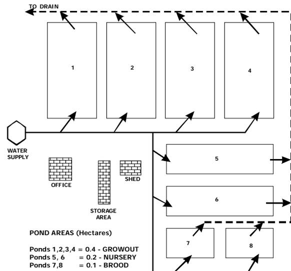
**Figure 6: A generalized layout of a fish farm showing ponds and support facilities, water supply and drainage systems**
