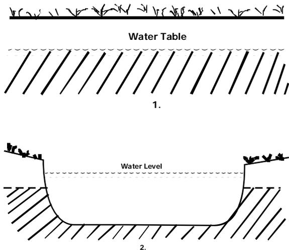
**Figure 4: Pond construction in swampy area**
