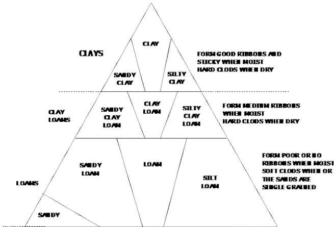
Figure 1: Textural triangle showing soil types and classifications for use in simple on-site testing.
