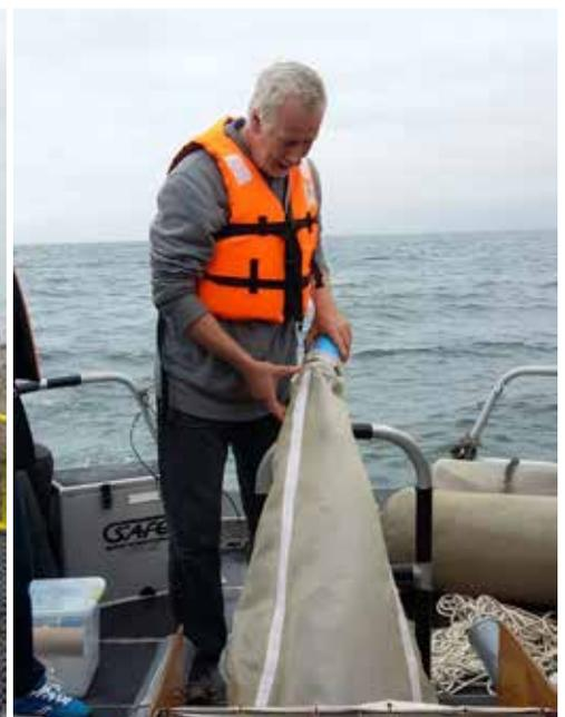
Researcher preparing sampler for microplastic sampling
